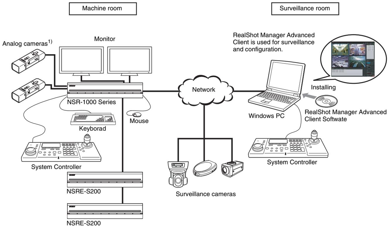
1) The NSR-1050H is standard equipped with an NSBK-A16 analog encoder board, but the NSR-1200/1100 requires an optional NSBK-A16 expansion.
